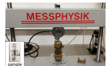
Fig. 4: Tensile testing machine
