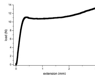
Fig. 5: Collected extension vs. load plot of a bundle of hair
