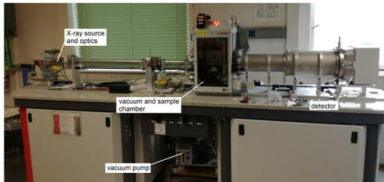
Fig. 2: SAXS-system of the Dynamics of Condensed Systems group
