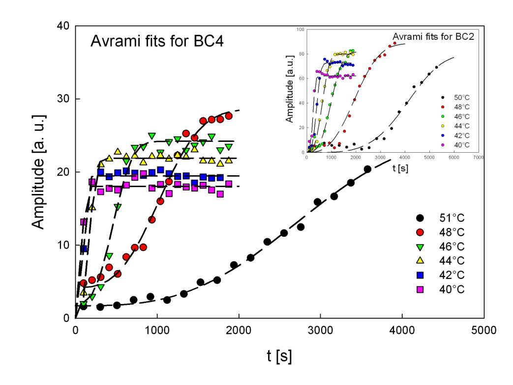
Avrami Fits at different temperatures for the BC4 sample (large graph) and the BC2 sample (small graph).
